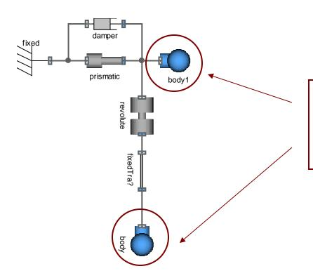
We have to set the gravitational acceleration twice, although it is actually a global constant.
