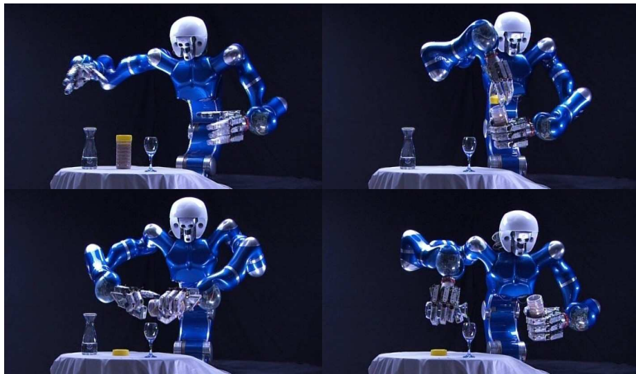
Fig. 1. DLR’s humanoid robot ‘Justin’ (upper body only) preparing a drink: after recognition of the scene unscrewing the lid from a jar of instant tea, dropping some grains of tea into a glass, and adding water from a carafe.
